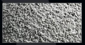
Nanobiocoat : 700µ porous coating + HAP
